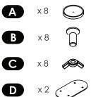
M6 x 20mm countersunk bolt M8 wing nut Cork isolator
