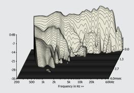
ABOVE: Panel resonances are well suppressed in this small box with only mild driver modes at 2kHz/6kHz
